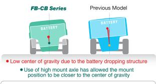
The small movement of the center of gravity during turning enables smooth and safe travelling.
